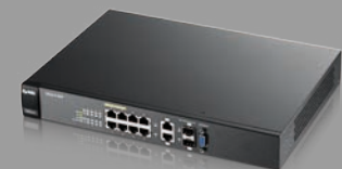
ZyXEL GS2210-8HP Managed Gigabit-Switch PoE+ (8x 10/100/1000 PoE, 2x Combo für SFP)
